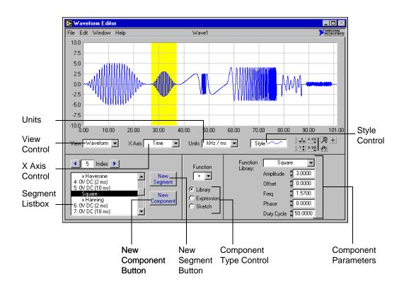
The Waveform Editor front panel of VirtualBench-Arb has the following features:
